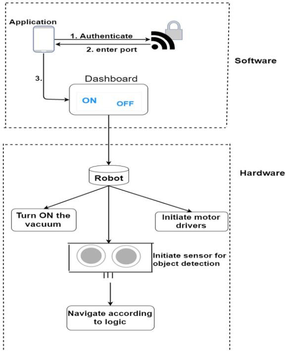
Figure.3: Architecture diagram of the Smart vacuum robot.
