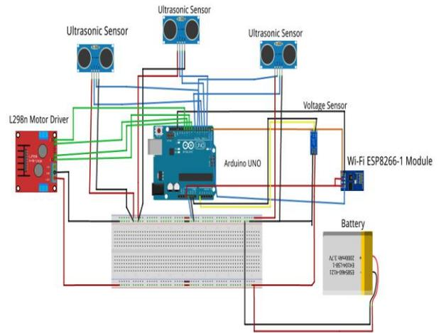
Figure.4: Circuit Diagram of Robot
