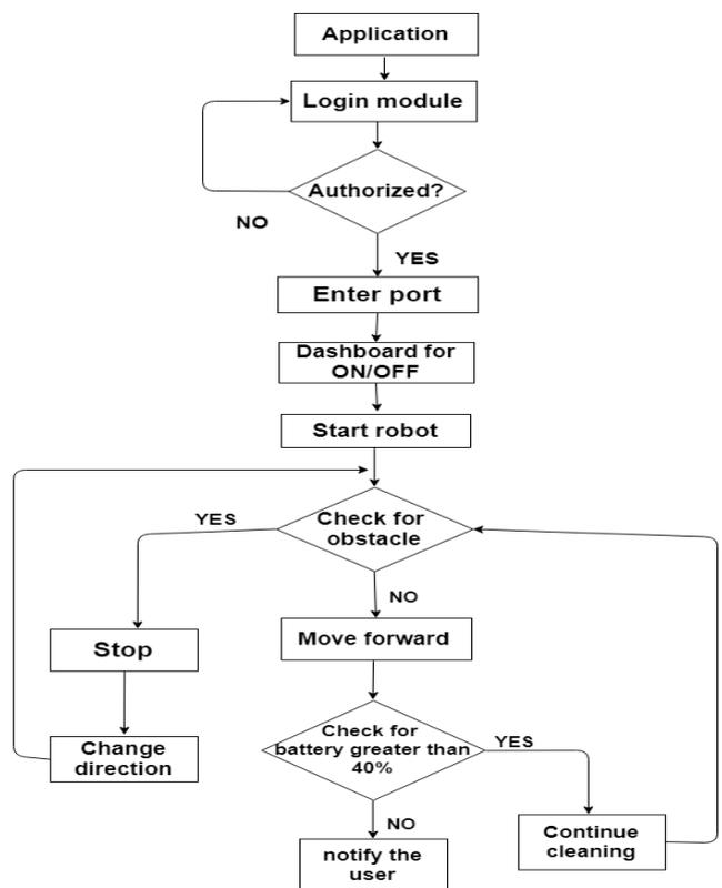
Figure.2: Flow diagram.
