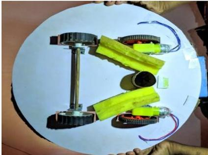
Figure.13: Vacuum Attached to the Robot.
